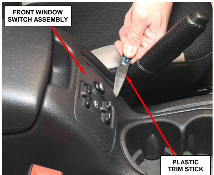
Figure 2 – Front Window Switch Assembly
