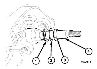
Fig. 1 \*\*WAVE WASHER, SHIM, AND LOWER BEARING WEDGE INSTALLATION\*\*
