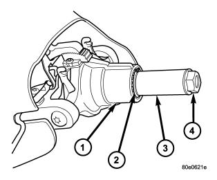
Fig. 2 SNAP RING INSTALLATION USING TOOL 05083385AA
