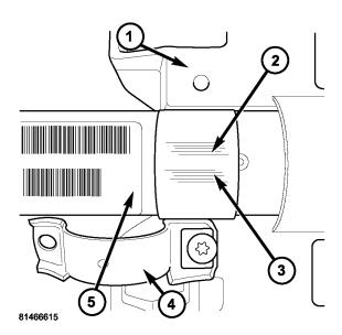
Fig. 3 APPLYING TAPE TO STEERING COLUMN
