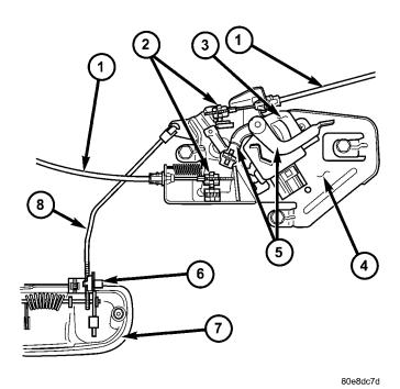
Fig. 1 LATCH CONTROL ASSEMBLY & HANDLE
